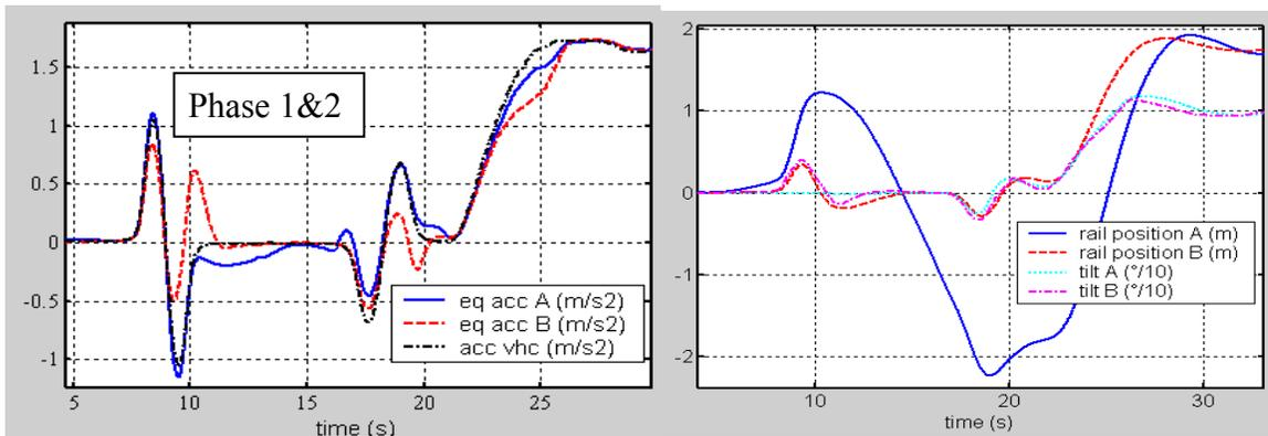
Figure 4: the driver performs a double lane change just before entering the curve
